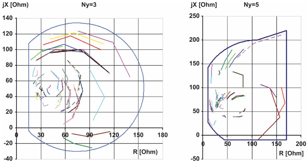
**Figure B.8—Examples of equivalent impedance areas based on a set of system conditions**
