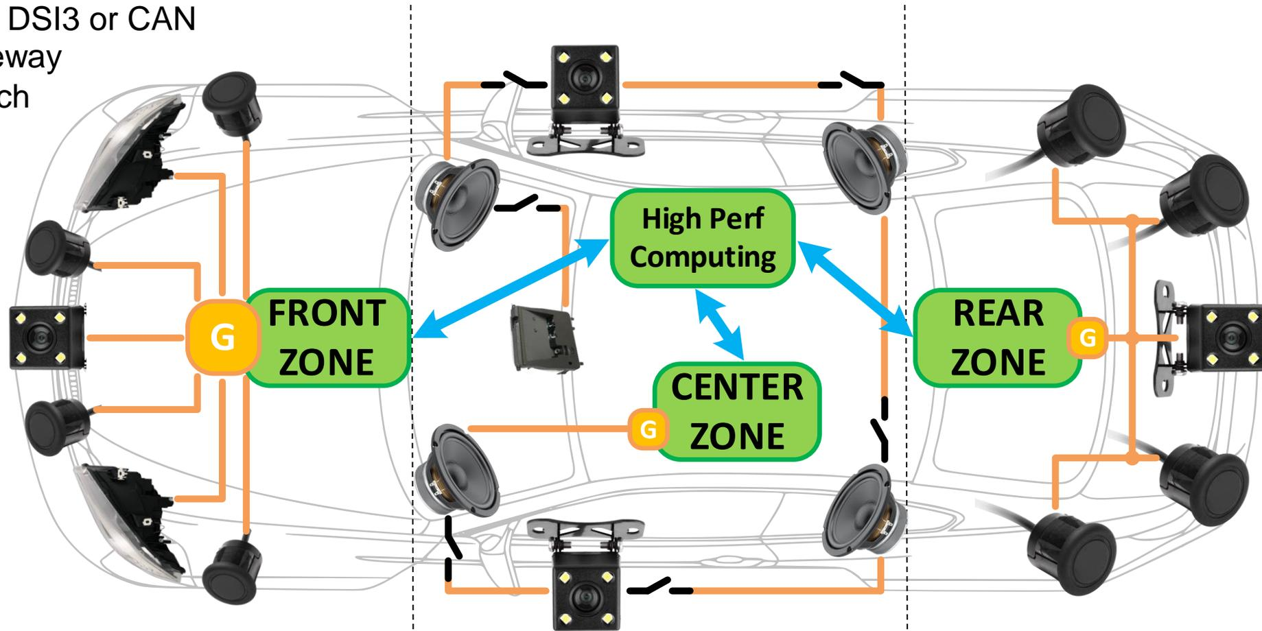
Hardware solution using point to point
