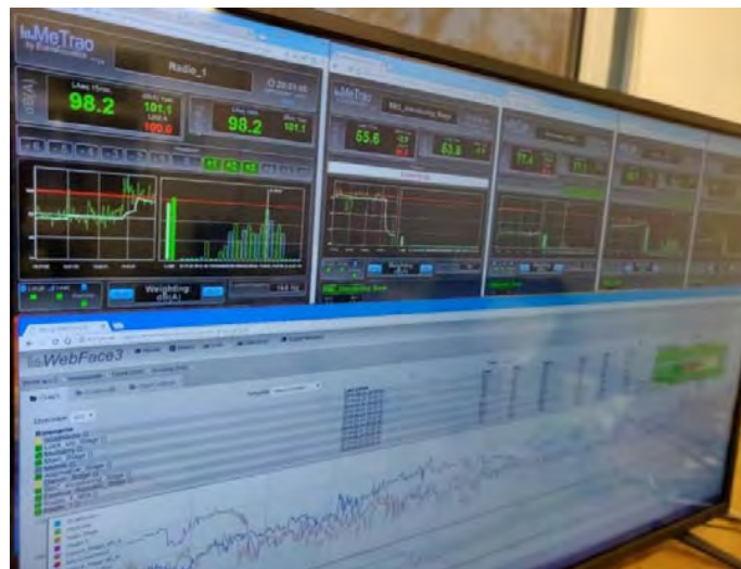
Figure 5.10 User interface for MeTrao Super-Correlator, used to identify source and frequency bands of noise issues at multiple stage festivals and to predict potential problems with noise pollution
