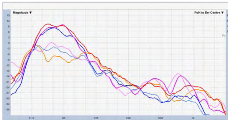
Figure 6.14 Measured results of sound pressure level distribution at three test points off-site, but on-axis to the primary system. The magenta, pink and dark blue traces are the primary system on its own, while the pink, light blue and orange are with the secondary system applied [353]
