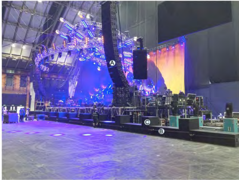
Figure 6.8 Primary sound system used for the listening tests including the main line arrays (A), the standard bandwidth subwoofers (b) and infrasound subwoofers (C) [109]
