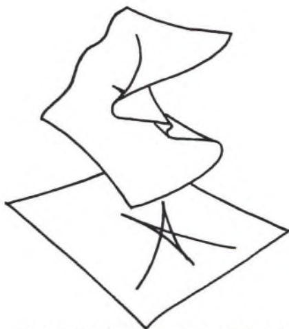
Fig. 4—In the later stages of development of the butterfly factor, the manifold develops a third inner sheet. The bifurcation set which this produces has the shape indicated in this sketch. The term "butterfly" is taken from the shape of this bifurcation set, which has been likened to that of an abstract butterfly.
