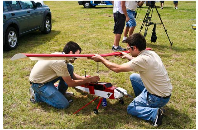
Removing the wing from the UAV and preparing to refuel.
