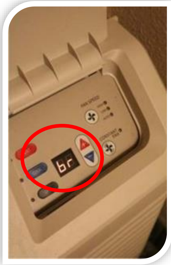
IMAGE: AC “BR” ERROR CODE INDICATING LOW VOLTAGE
