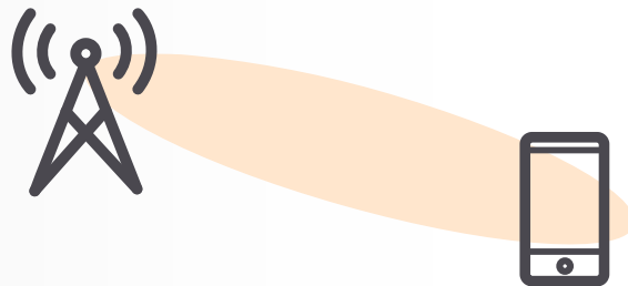
Beamforming to increase received power and SNR
