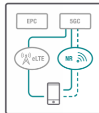
OPTION 4A: Non-Standalone eLTE, NR assisted, 5GC connected
