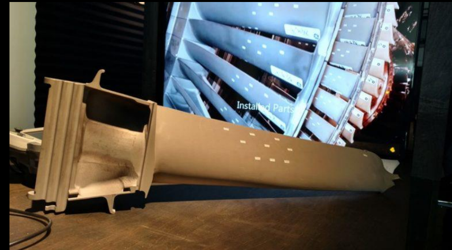
Turbine blade with printed strain sensors. Source: Optomec
