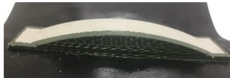
8 to 12 GHz Conformal Phased Array Antenna. 64 elements. Improving RF designs.
