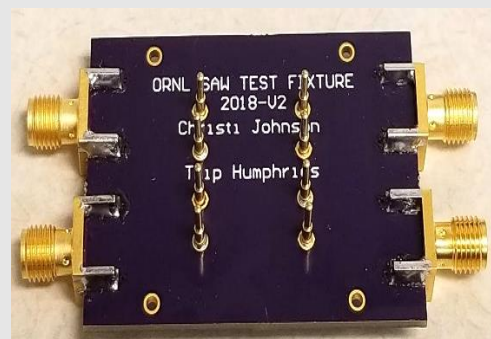
Pogo pin connections (no wire bonds)
