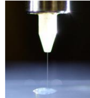
Contactless, Fine Feature Printing Process
