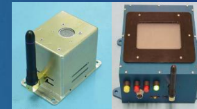
Wireless Oxygen Sensor With Hub for Possible International Space Station Environmental Applications
