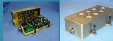
Fire Detection/Environmental Monitoring System for possible Space Craft Habitat Applications (Wireless Design Available)
