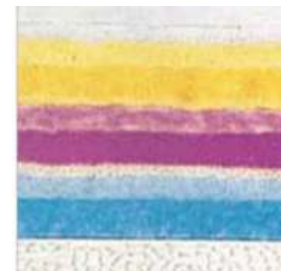
Film structure Source: Kodak
