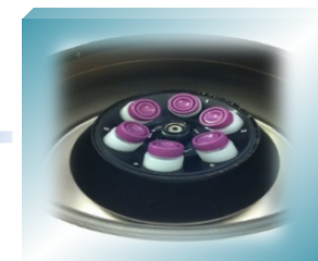
Centrifuging to remove unexfoliated particles
