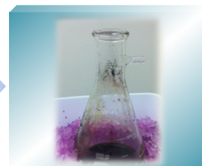
Oxidization using \text{KMnO}_4
