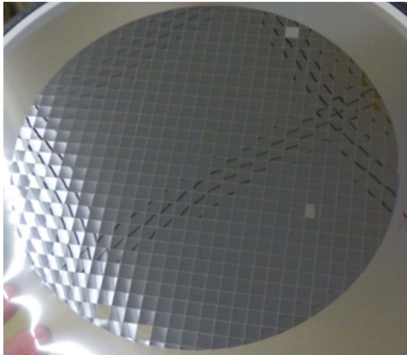
Thinned wafer at expansion step
