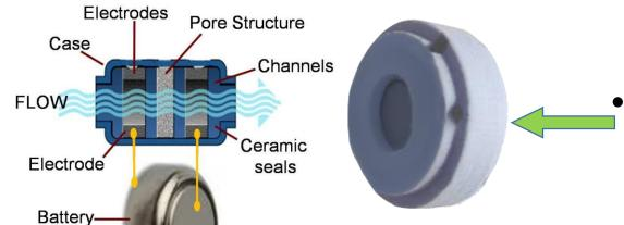
Electrophoretic pump for micro fuel cells
