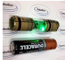
Any device can have its internal battery charged in the vicinity of the emitter pad
