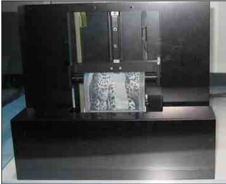
Flexible LCD display at the Philips Electronics booth. The roller moves up and down rolling up the display while an image is displayed.
