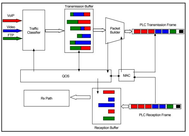
The service classifier is designed to differentiate between 8 types of traffic.
