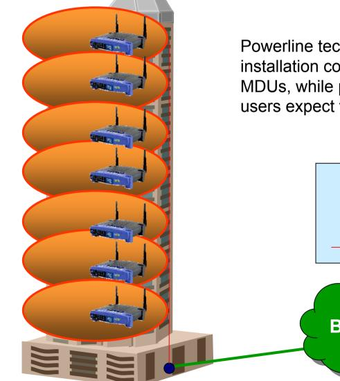
Powerline technology almost eliminates the installation costs for Wireless networks in MDUs, while providing the convenience that users expect from Wireless
