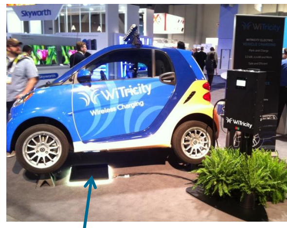
Witricity Wireless charging pad via electron magnetic resonance
