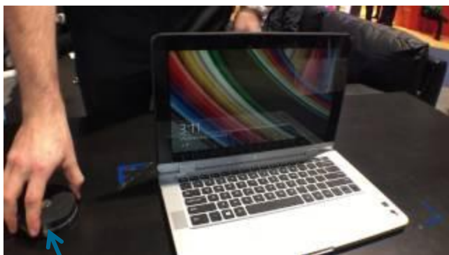
Laptop powered by Witricity charger mounted under the table
