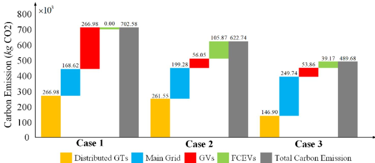
Fig. 3. Carbon emissions of the coupled system in three cases.
