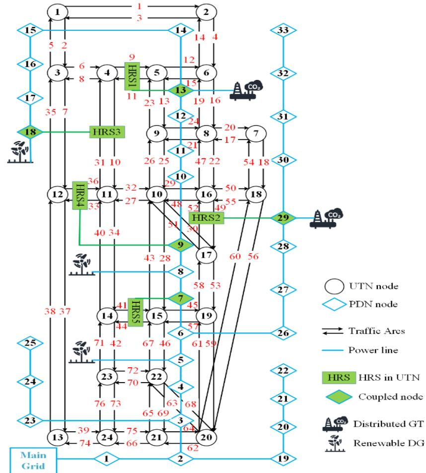
Fig. 2. Topology of the hydrogen-integrated UTN and PDN in Sioux Falls city.
