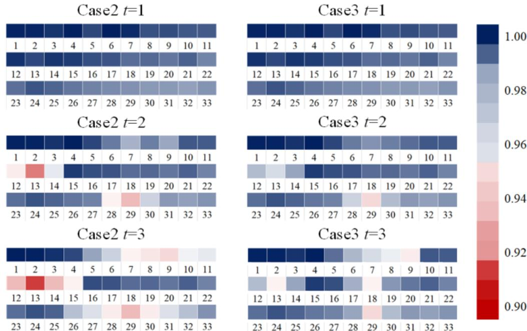
Fig. 5. The voltage magnitude distribution of all buses in PDN.
