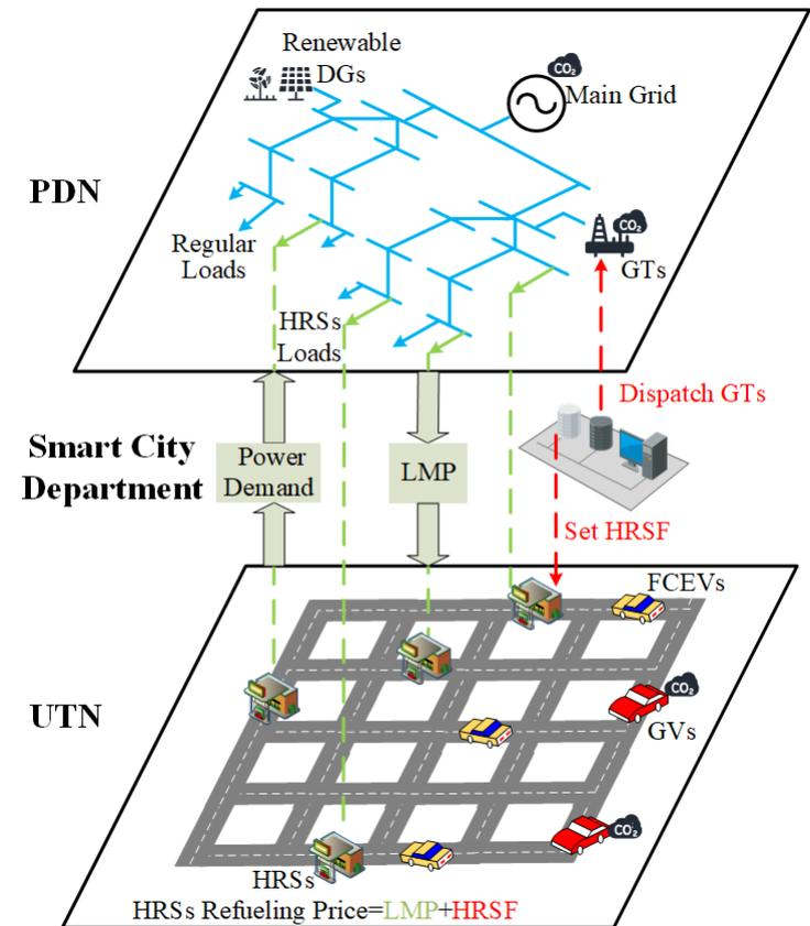
Fig. 1. HRSF based coordinated operation framework of hydrogen-integrated UTN and PDN.
