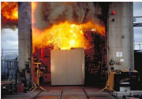
Fig. 3. Medium-Voltage Arc Resistant Switchgear Under Test.
