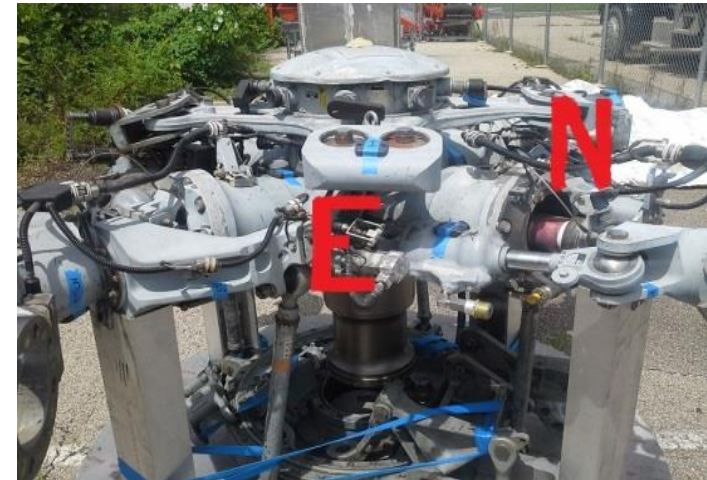
Rotor-head assembly with RFID tag placement
