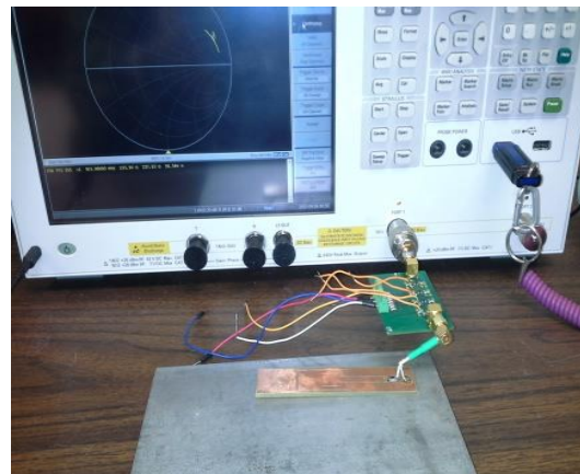
CASE 2: Metallic object attached to antenna
