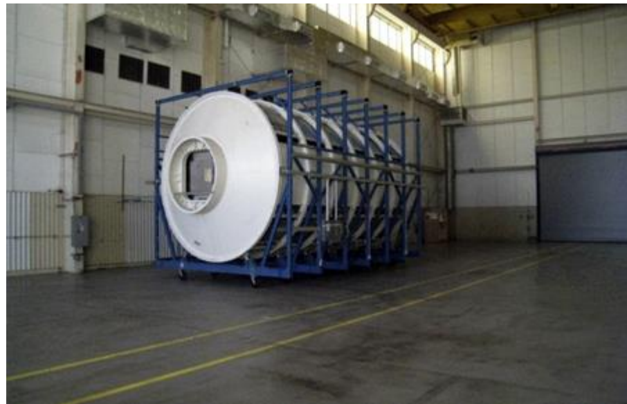
Habitat mock-up previously developed at KSC and now at MSFC. New habitat will be similar.
