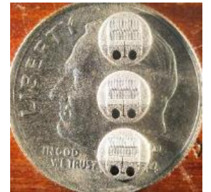
3 Model 141 sensors on a US dime
