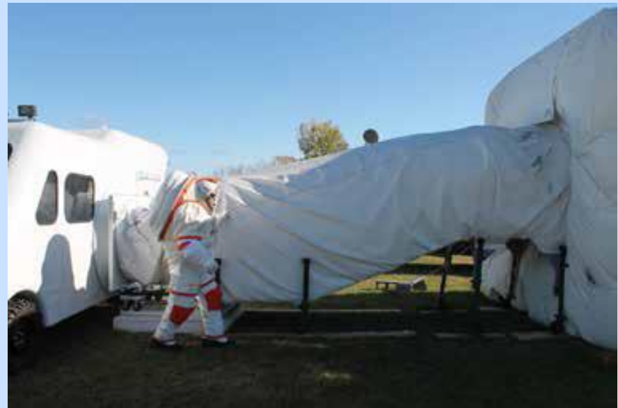
A researcher at the University of North Dakota completes a routine examination of integrated system of inflatable habitat, docking tunnel, and electric rover during 30-day stay in a Lunar/Martian analog mission..
