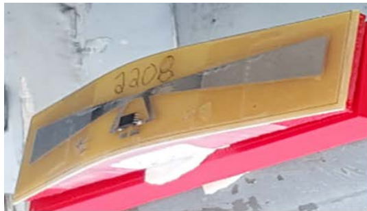
Curved bowtie antenna (left), mounted on rotorhub for testing (right)
