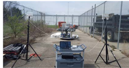
Basic T-matched bowtie antenna (left), and experimental test bed on H-60 rotorhub (right)
