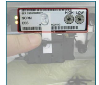
Example Rotary Coding Switches
