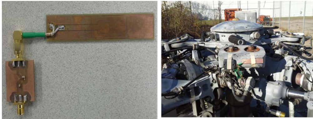
ISN with patch antenna (left) and the tag on rotorhub test bed (right)
