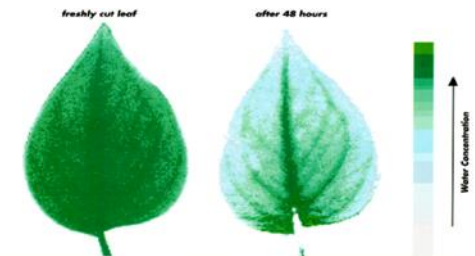
Plate II. Left: THz image of a fresh leaf. Attenuation of THz radiation through the leaf is largely due to water within the leaf. Right: THz image of the same leaf after 48 h. Water has clearly evaporated from the leaf, except from the stems of the leaf. At the far right is the color scale indicating the relative water concentration within the leaf; darker green corresponds to higher water concentration.
