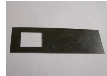
Shadow mask fabricated with UV Nd:YAG laser on stainless steel 0.2mm-thick foil
