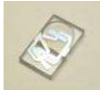
Pressure sensor chip
