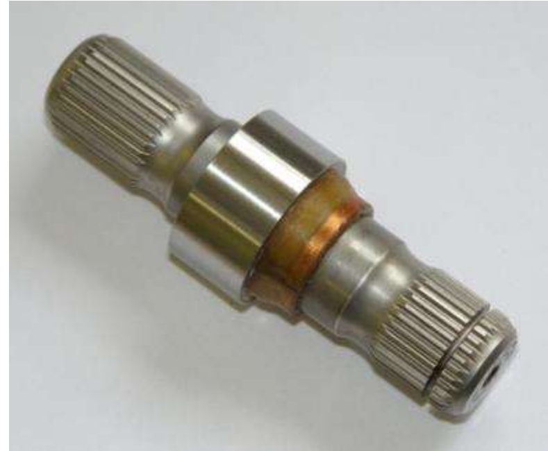
Assembled torque transducer
