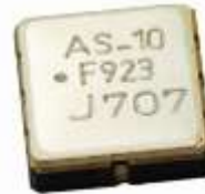
Packaged temperature sensor TSE AS10
