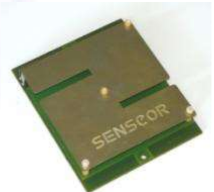
PIFA antenna mounted temperature sensor TSA D003
