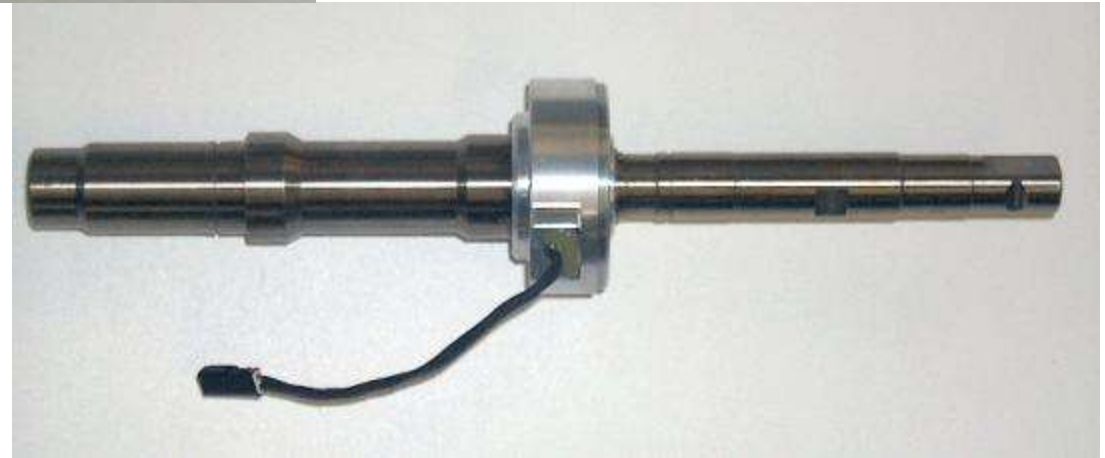
EPAS torque sensor installed on a steering shaft with a pinion
