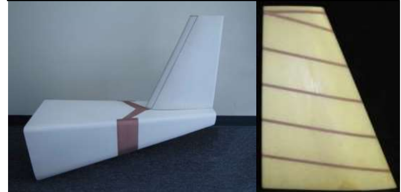
Integrated VHF/GPS for Dakota UAV Platform
