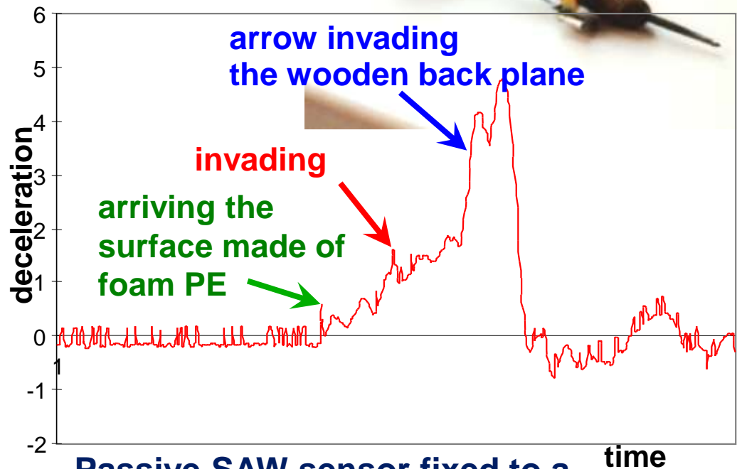
Passive SAW sensor fixed to a dart arrow, invading the target
