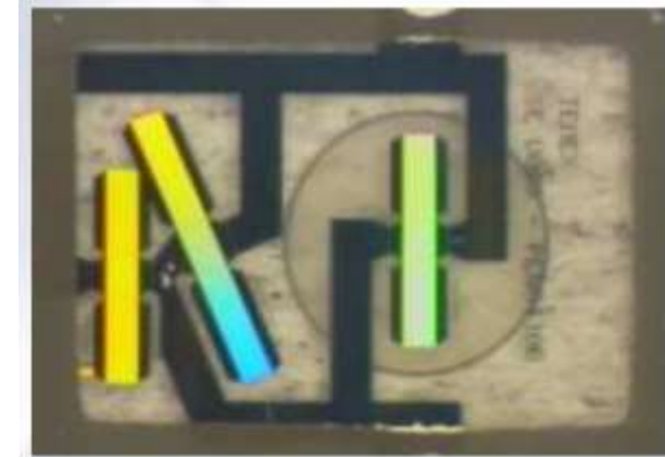
pressure & temperature sensor (8x4mm)
