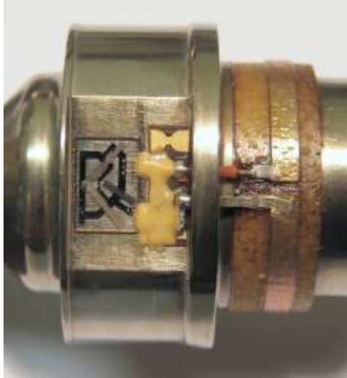
The KERS shaft with the bonded HFSAW sensing element
