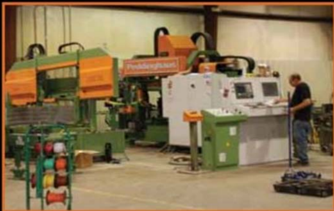
◀◀ A new Peddinghaus structural drill in the stringer cell area.
