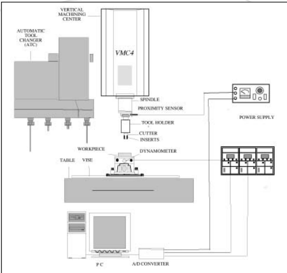
**Figure 3. An example of cutting force signal converted as collectable digital data.**
