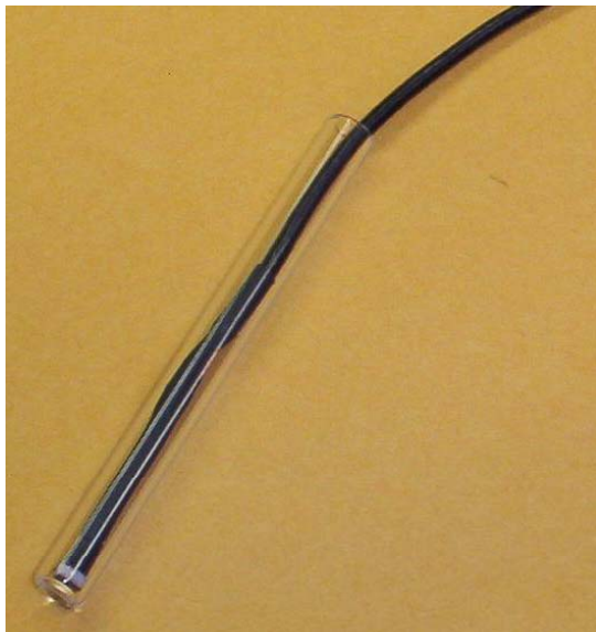
Figure 3. The SALS sensor and controller box. The CdS photocell is encapsulated in a glass tube with a flat bottom window. An insulated cable connects the photocell to the controller box (right)
