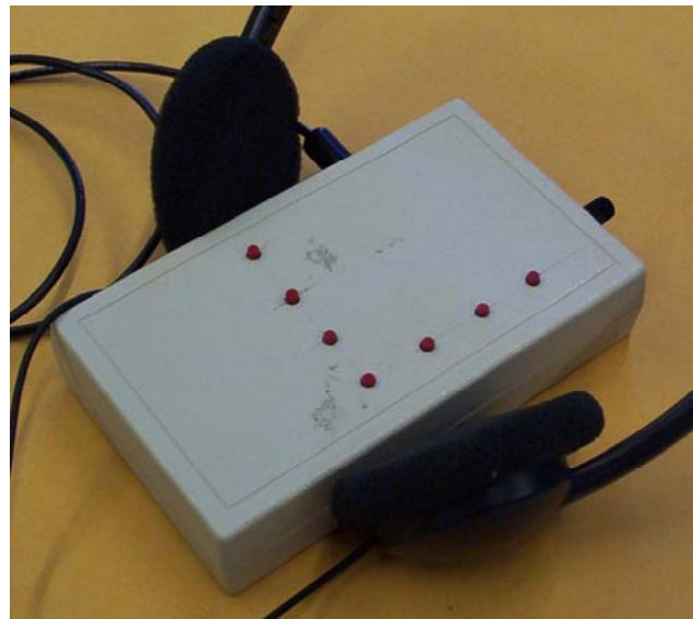
Figure 3. The SALS sensor and controller box. The CdS photocell is encapsulated in a glass tube with a flat bottom window. An insulated cable connects the photocell to the controller box (right)
