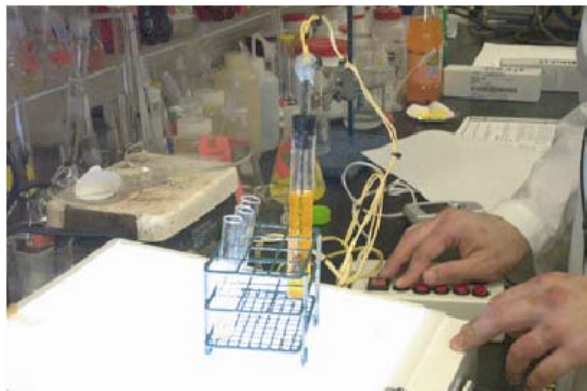
Figure 1. Monitoring a color change in a chemical reaction using the SALS and a light box.
