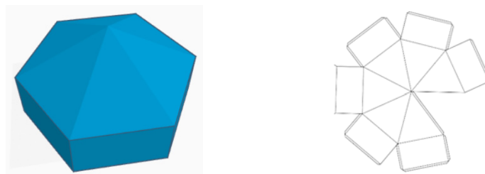
Figure 5. Design of the Canopy at Tinkercad and Its Development at Pepakura
