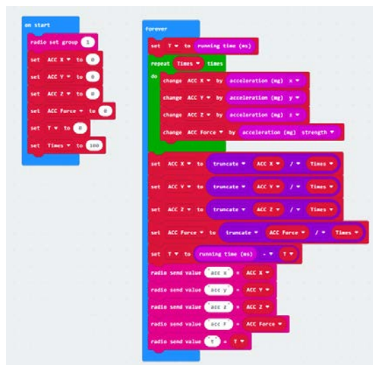
Figure 11. Program of the Transmitter micro:bit
