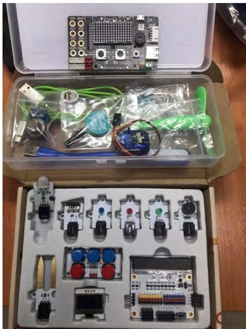
Figure 12. KidBright and Ultrasonic Sensor kit (Top left) for detecting the movement of objects
