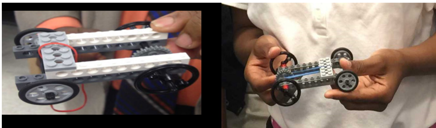
Figure 3. Experiment 3: The two figures display two different rubber band cars built using the alternative parts (more gears, bigger wheels, rubber bands with different elasticity, etc.). These are examples that were designed and built by the students.
