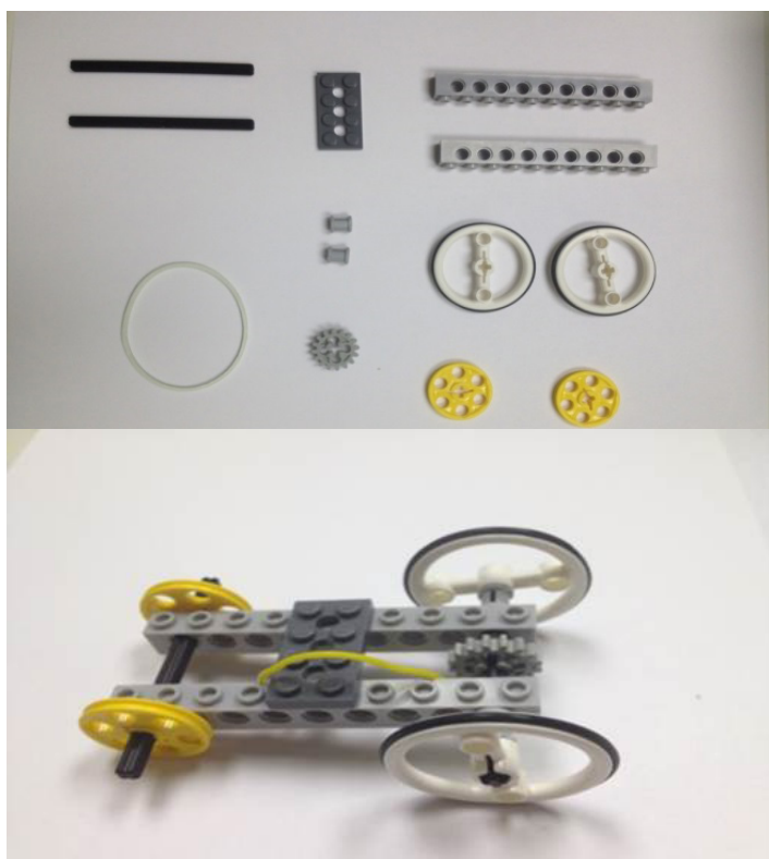
Figure 2. Experiment 2 consisted of building an initial rubber band Lego car using the parts shown in 2A. 2B shows the fully assembled basic Lego car.
