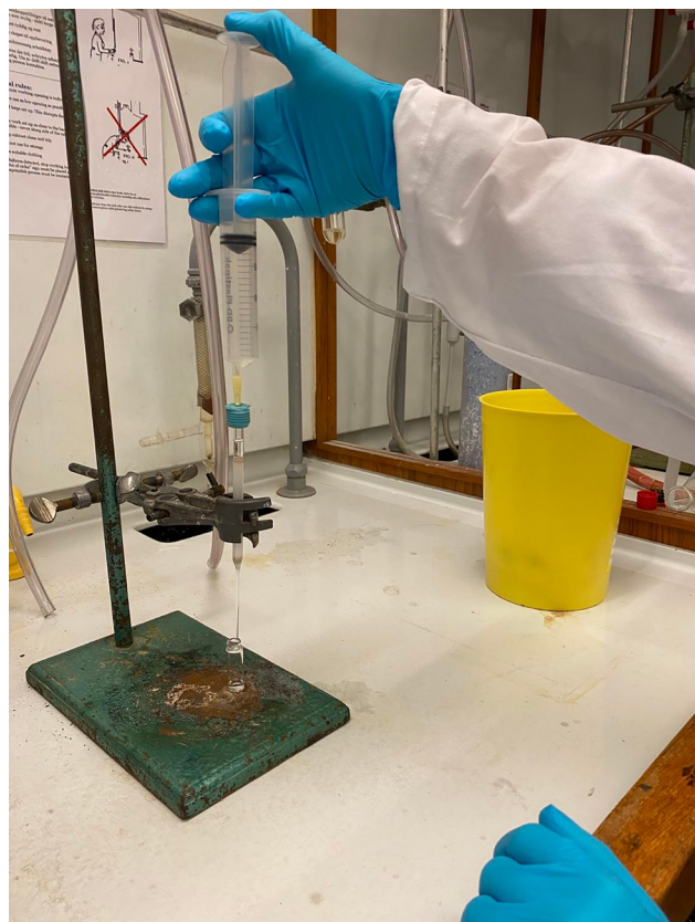
Figure 3. Eluting the column using a syringe fitted with a septum.
