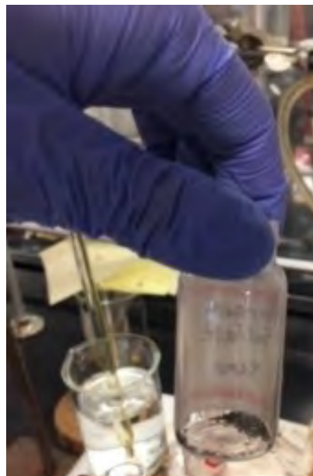
FIGURE 11: Ferrous Sulfate decomposing at approximately 86 °F
