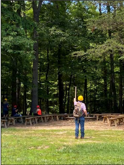
Tree Measurement with a Biltmore Stick
