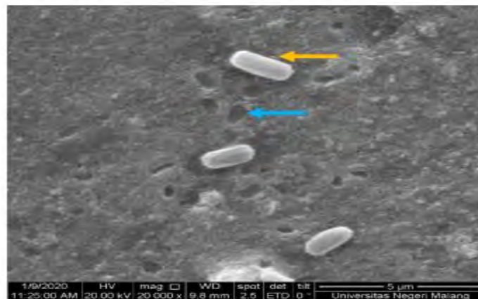
Figure 2: Electron micrograph of soil bacteria Styrofoam degradation Remarks: Damaged Styrofoam surface (Blue) dan Styrofoam-degrading bacteria (Orange).
