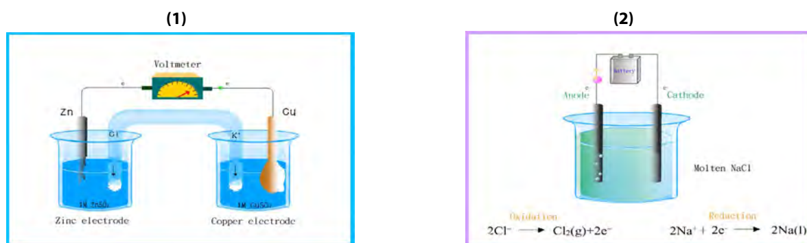
Figure 2. The two animations integrated into ACM in (1) Galvanic cell, and (2) Electrolysis of \text{NaCl}_{(l)} .
