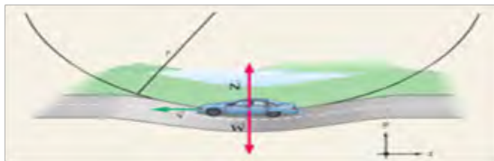
Figure 7: A car crosses the road on a decreasing radius with a radius of 65.0 m depth
