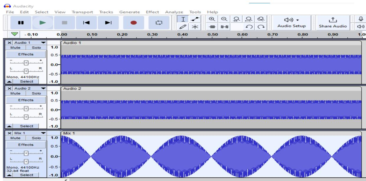
Note. The Bottom Track Shows 5 Beats in a Timeframe of 1 Second. The Number of Beats in a Span of One Second is Attributed to the Frequency Difference Between Two Sine Waves (i.e.,  $505 - 500 = 5$  Hz).
