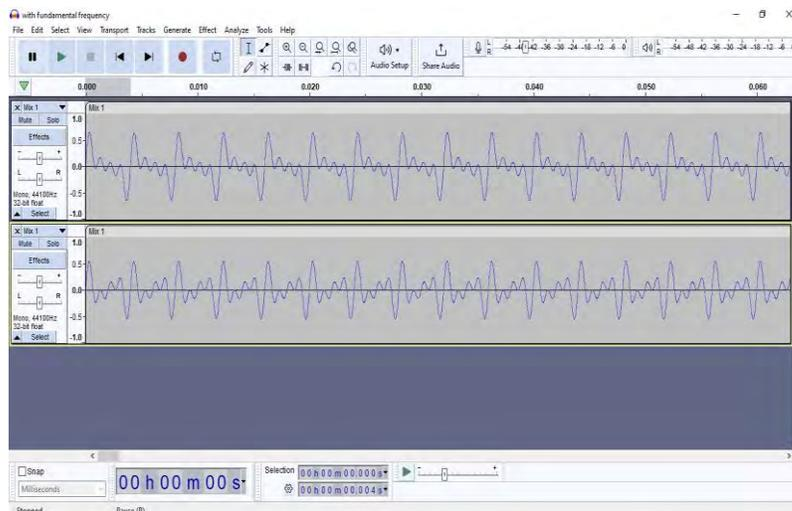
Step 10 The figure above clearly shows that the period and wavelength of both waveforms are the same. To exclusively listen to the first track (“with fundamental frequency”), mute track 2 (“without fundamental frequency) and then press the Play button. Subsequently, track 1 should be muted while deactivating the Mute button on track 2. At this point, track 2 can be played independently. After playing these two tracks separately, users will perceive that both waveforms have the same pitch.
