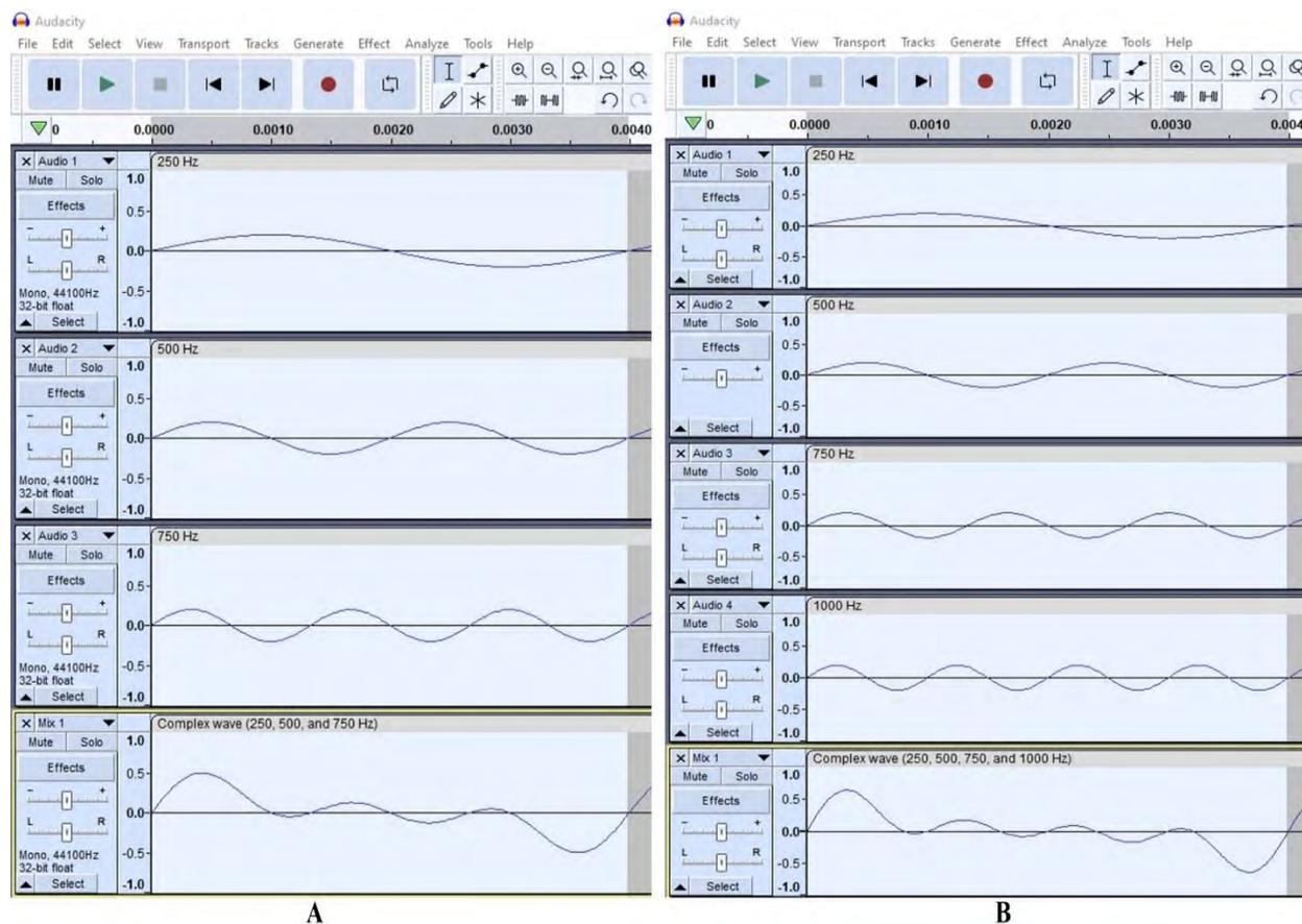
Note: **Panel A** illustrates sine waves of frequencies 250, 500, and 750 Hz and the resultant complex wave (bottom track). **Panel B** illustrates sine waves of frequencies 250, 500, 750, and 1000 Hz and the resultant complex wave (bottom track).
