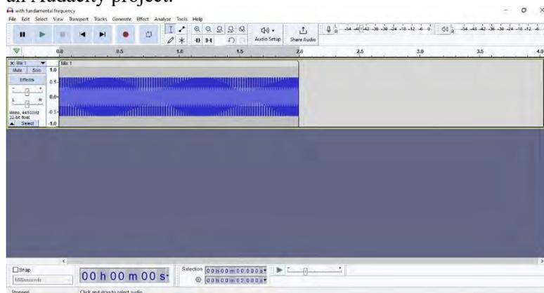
Step 4 Use the existing window of Audacity and select Edit > Undo Mix and Render to return to the original four harmonics/waveforms.
