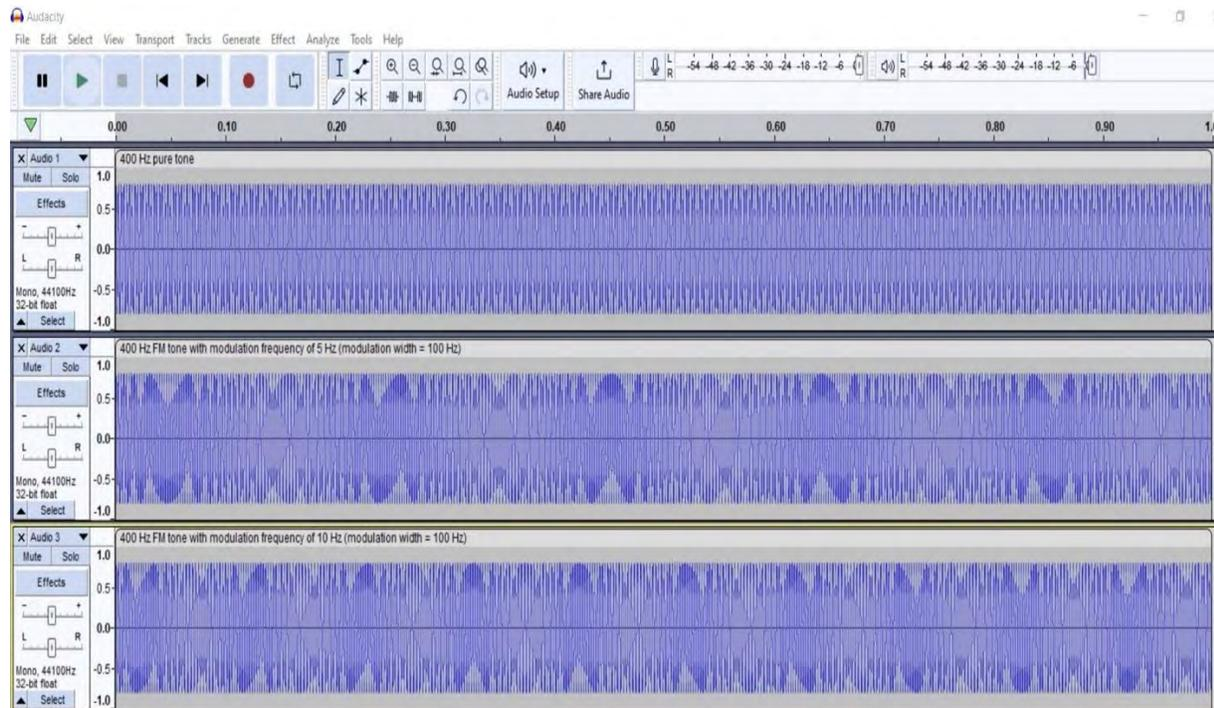
Note. The second and third tracks represent 400 Hz frequency modulated (FM) tones with modulation width of 100 Hz and modulation frequency of 5 and 10 Hz, respectively.
