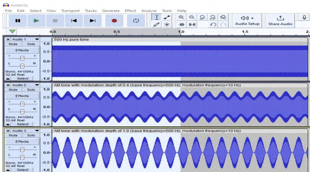
Note. The second and third tracks represent 500 Hz amplitude modulated (AM) tone with a modulation frequency of 10 Hz, and modulation depth of 0.4 and 1, respectively.
