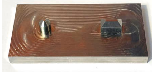
Figure 5. Machined functional gauge used for position of hole and slot inspection method.
