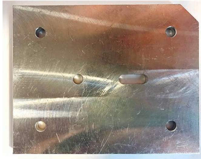
Figure 3. Machined Part B with hole and slot and four corner holes.
