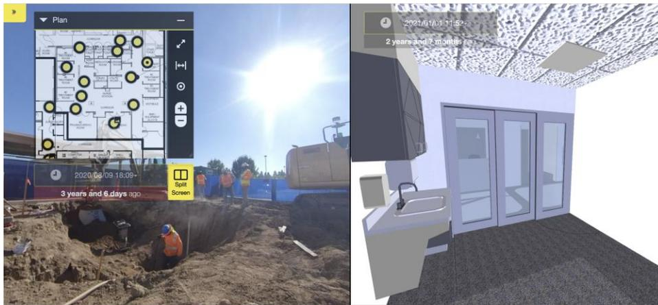
Figure 3. A SplitScreen View of the VFT Displaying an Active Construction Site Scene and a 3D Model Scene
