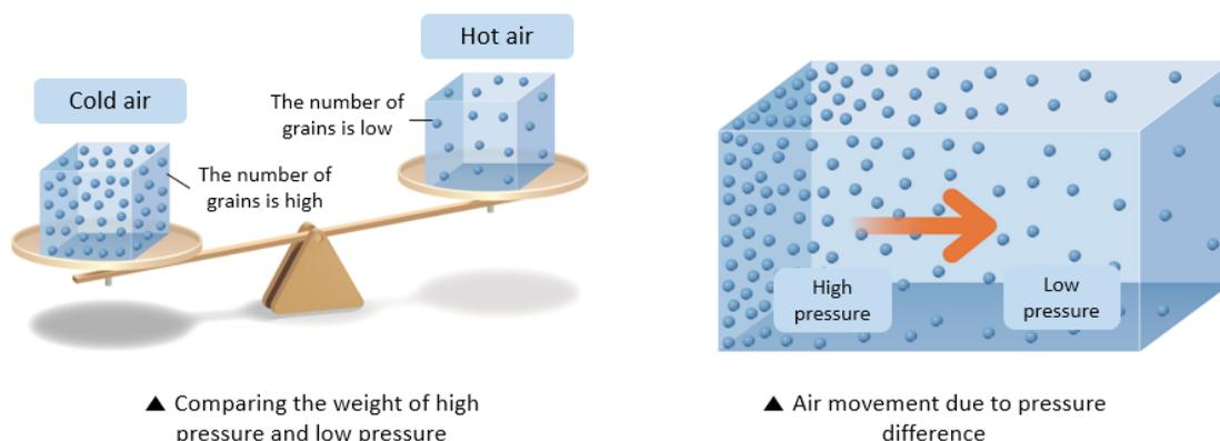
▲ Comparing the weight of high pressure and low pressure
