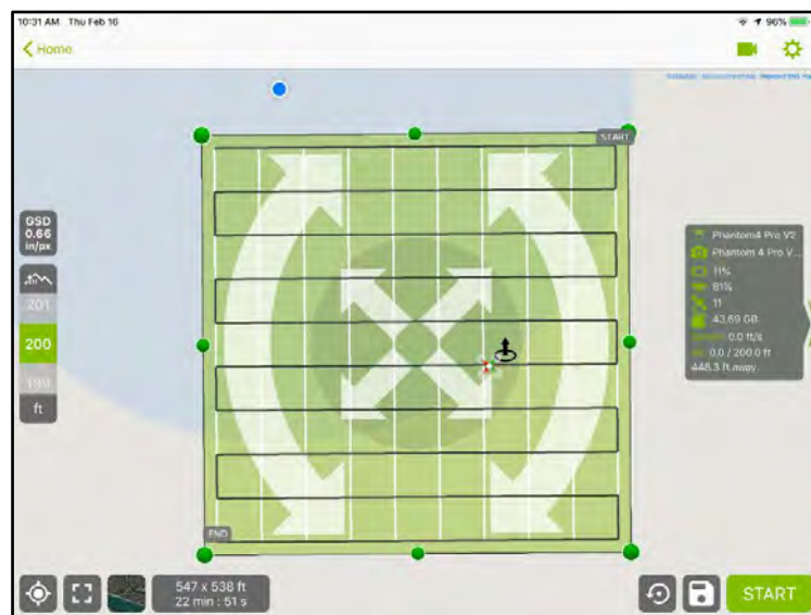
Figure 1. Example of a drone flight path depicting 80 percent overlap and 80 percent sidelap flight lines for orthophoto mosaic creation
