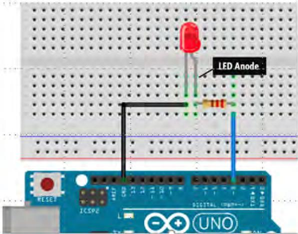
**Activity:** Use the pin connector wires, resistor, and LED to "breadboard" the circuit as shown in the drawing.
