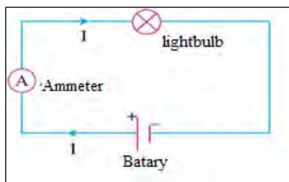
**Figure 1.** Circuit Drawn on the Board
