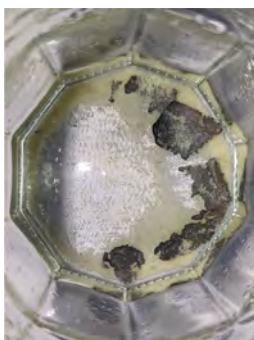
Figure 3. Crystals (white) and corroded Al foil (grey) obtained upon drying of the suspension resulting from the CO 2 reduction with Al
