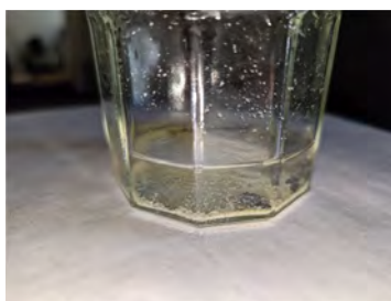
Figure 2. White precipitate obtained from the bubbling of \text{CO}_2 on an activated Al surface
