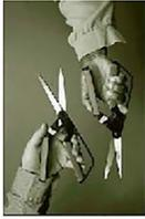
Large-grip scissors accommodate use with either hand and allow alternation between the two in highly repetitive tasks.
