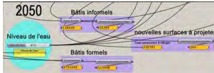
Figure 3: Parametric model evaluating the flooded surfaces in the district of El-Harrach in Algiers, the number of people to be rehoused and the new surfaces to be built according to the rise of water.
