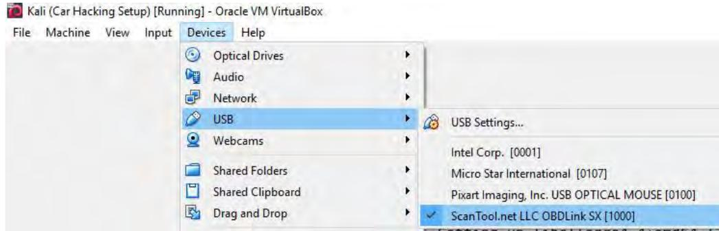
Figure 9: You can connect a physical OBD-II to USB cable to your virtual machine in VirtualBox by going to the virtual machine's menu and selecting **Devices > USB > ScanTool OBDLink** (or the name of your OBD-to-USB cable).
