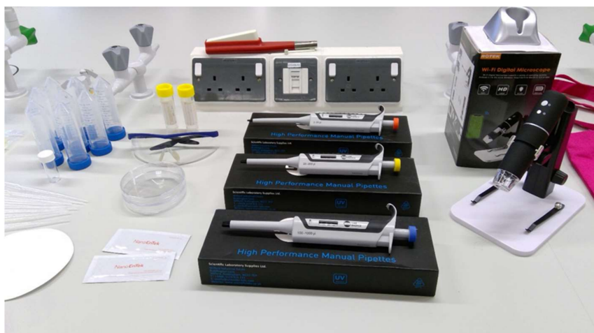
Figure 1. Essential equipment and consumables that formed the basis of the Bioskills at home kit including micropipettes of three assorted sizes (centre) and a digital microscope.
